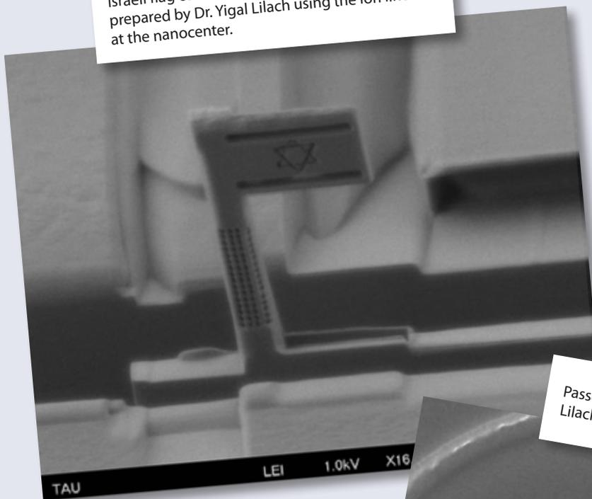
Passover plate, curved in silicon by Dr. Yigal Lilach using the Ion line FIB at the nanocenter.
