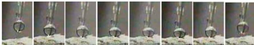
Fig.2 Camera snapshots. Time interval between the pictures is 200ms. 2 $\mu\text{l}$  water drop cannot be detached from the pipette and placed on a irradiated ZnO powder superhydrophobic surface.
