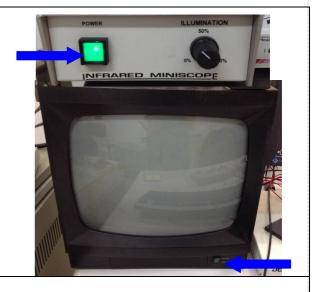
Pull the rod down and slide it in completely (look on TV screen to see that the sample holder reaches the right place)
