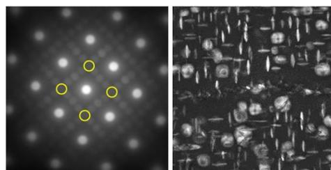
Figure 2 : Grain boundary and precipitates in a Ni-based super alloy generated from an EMPAD 4DSTEM dataset. (200kV) Sample courtesy: Prof.
