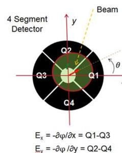
Figure 1: Segmented ADF detector illustrated with principle of DPC contrast
