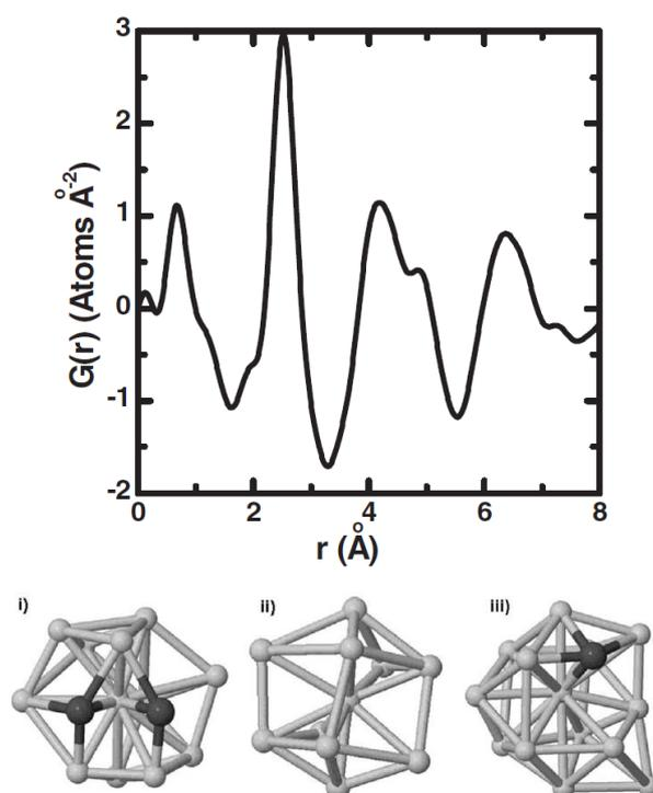
Fig.1, *Phys. Rev. B* **79**, 014203 (2009): (top) Example of a reduced density function,  $G(r)$ , of an amorphous ferromagnetic  $\text{Co}_{40}\text{Fe}_{40}\text{B}_{20}$  thin film. The peak positions correspond to characteristic bond lengths in the material.
