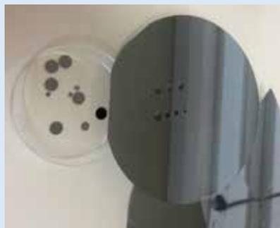
Milimeter in size silicon wafers – curved out by Dr. Yigal Lilach, using our new Laser Micromachining system
