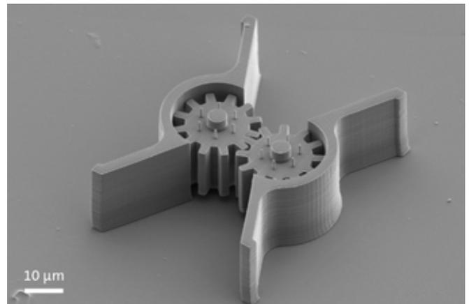
**Figure 2:** Micro Rapid Prototyping - Micro-gear for applications in micro rapid prototyping
