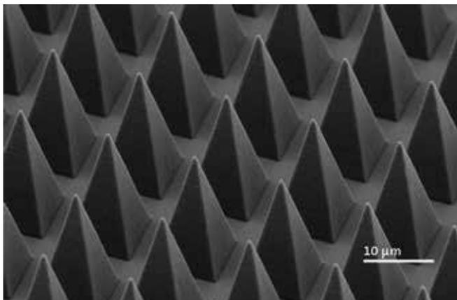
**Figure 3:** Micro-optics: Pyramid array for applications in micro-optics
