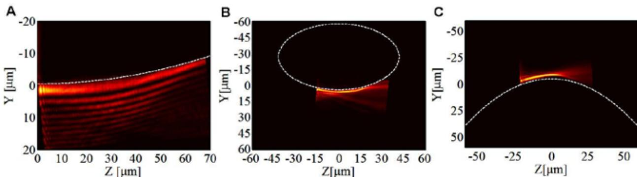
**Figure 4:** Measurements of plasmonic Airy, Mathieu and Weber beams. (A) Plasmonic Airy beam, (B) Plasmonic Mathieu beam, and (C) Plasmonic Weber beam. The white dashed line in all figures represents the designed analytical trajectory of acceleration.
