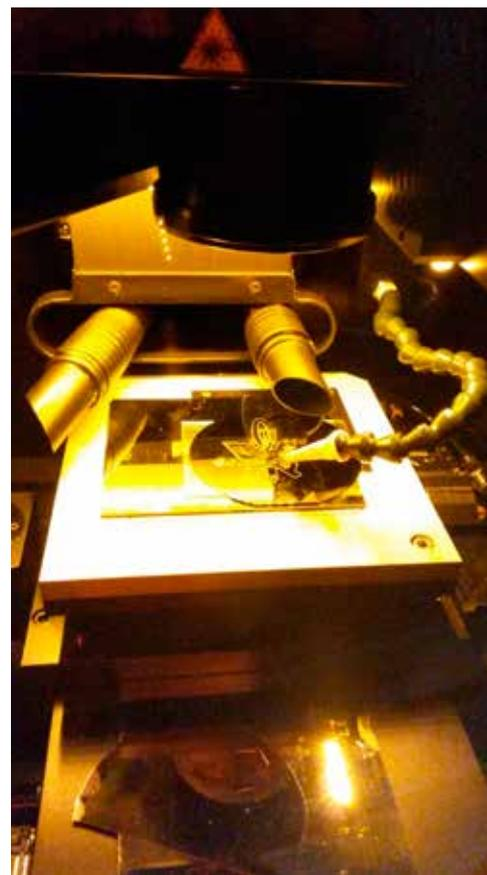
**Figure 2:** The Laser Micromachining in action: curving TAU symbol in silicon
