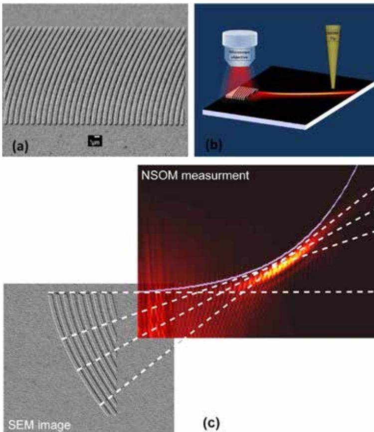
**Figure 3:** (a) SEM image of the fabricated binary plasmonic phase mask for the case  $Y=az^{1.5}$ . (b) Experimental setup. (c) Geometrical representation of the construction of a caustic SPP. Geometrical rays (white dashed lines) emanating from the two-dimensional plasmonic binary phase mask (a SEM image) which generated the caustic SPP (NSOM measurement). The mask and the measured SPP are for the case of an exponential trajectory (a solid purple line shows the analytical curve) [7].
