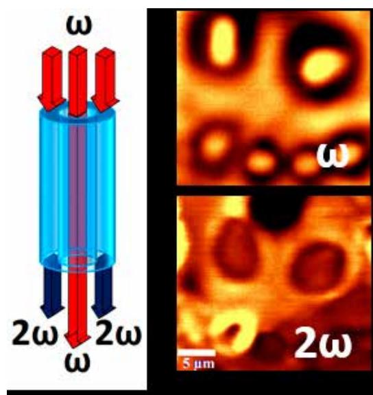
**Figure 2:** Illustration of the fundamental and second-harmonic generated wave (red arrows – fundamental wave, blue arrows – SHG wave), top: Linear waveguiding of FF peptide nanotubes, bottom: Non-linear waveguiding of FF nanotubes
