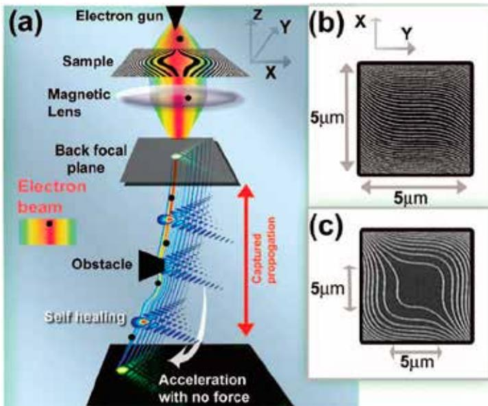
**Figure 2:** Setup for generating electron Airy beams [5]. The electrons are emitted from the field emission gun, pass through the nanoscale hologram and Fourier transformed using a magnetic lens. The desired electron beam is obtained at the back focal length, and it can then propagate to the slow-scan camera. (b) and (c) are two examples of masks that were produced for generating the electron Airy beams.
