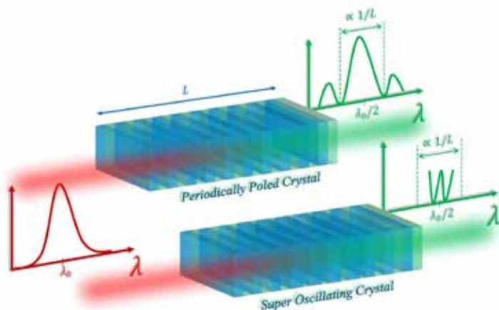
Figure 1. Schematic description of periodically poled and super-oscillating crystal
