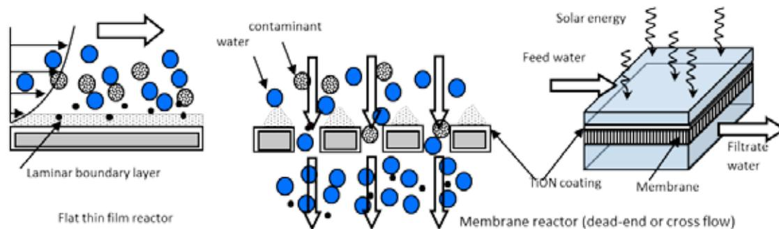
**Figure 1:** The principle of flat thin film compared to combined filtration and chemical degradation reactors
