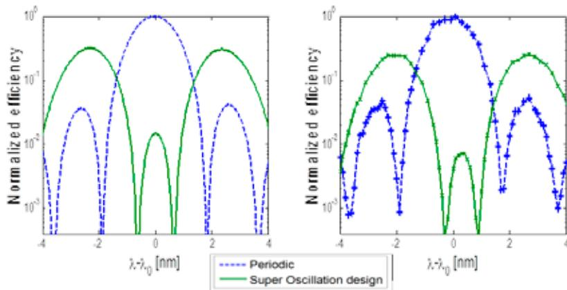
Figure 2. Normalized Efficiency. Simulation (left) and experimental (right) results of normal periodically poled (dashed blue) and super oscillating (solid green) KTP crystals. Both crystals have the same length of 10 mm, but the super oscillating crystal has a spectral width of only 1.1 nm (in green), 69% less than the spectral width of a normal crystal (in blue)
