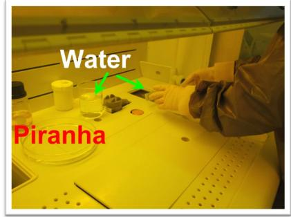
Leave the water running and start spilling the Piranha SLOWLY to the sink while diluting it with running water.
