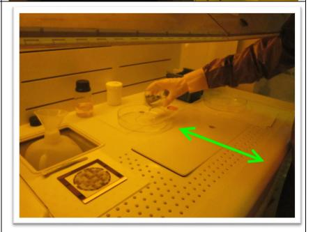
Take the sulfuric acid. Check the label!!! Carefully pour the sulfuric acid (150ml) into a different 8 measuring cup or rinse well the previous cup you used. You do not want to start the reaction yet! Clean the bottle neck and 9 bottom, and the bench from acid drops. Return the bottle to the cabinet.
